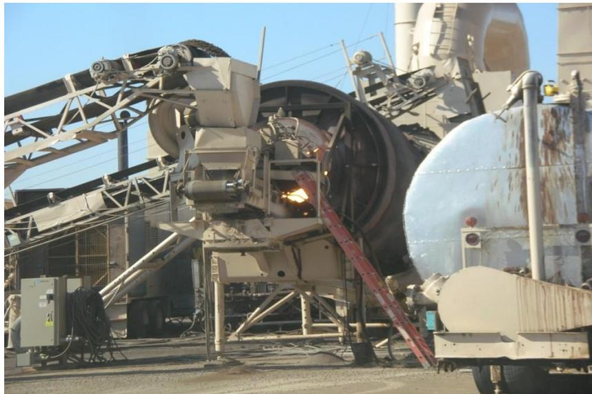
Figure 400.4 – Parallel-Flow Mixing Drum
