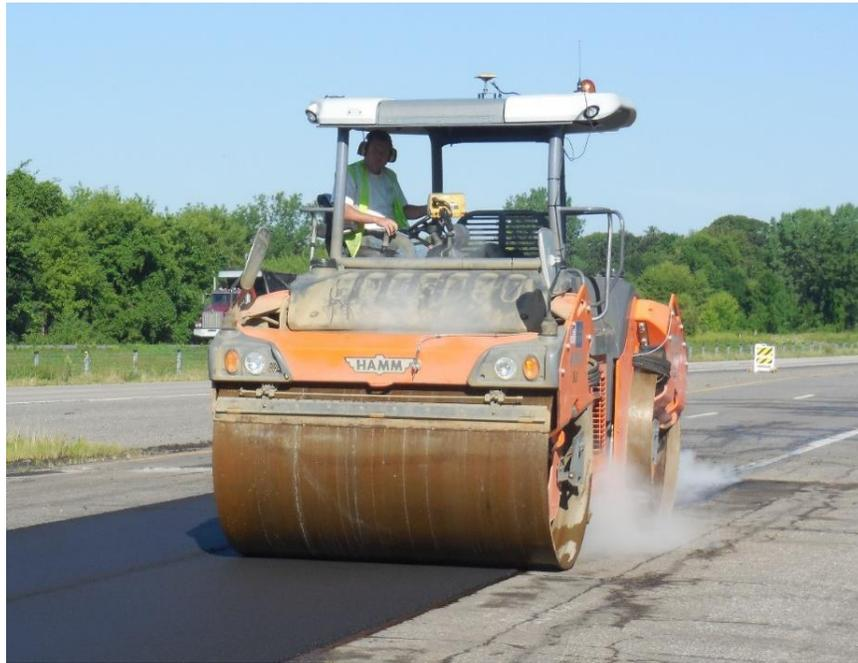
**Figure 500.18** – Vibratory Double Steel Drum Breakdown Roller
