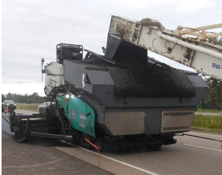
**Figure 500.17** – Spray paver in action. Note the tack coat spray bars in front of the screed.
