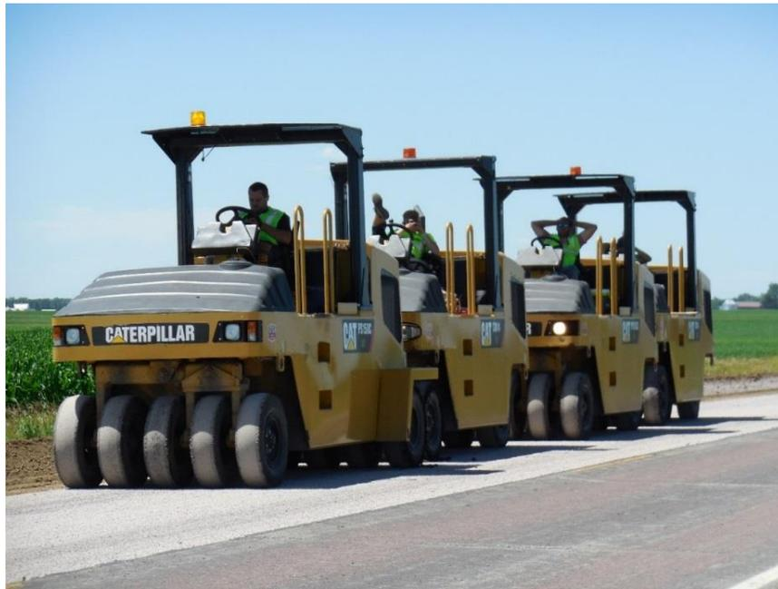
Figure 500.19 – Pneumatic Tired Rollers.
