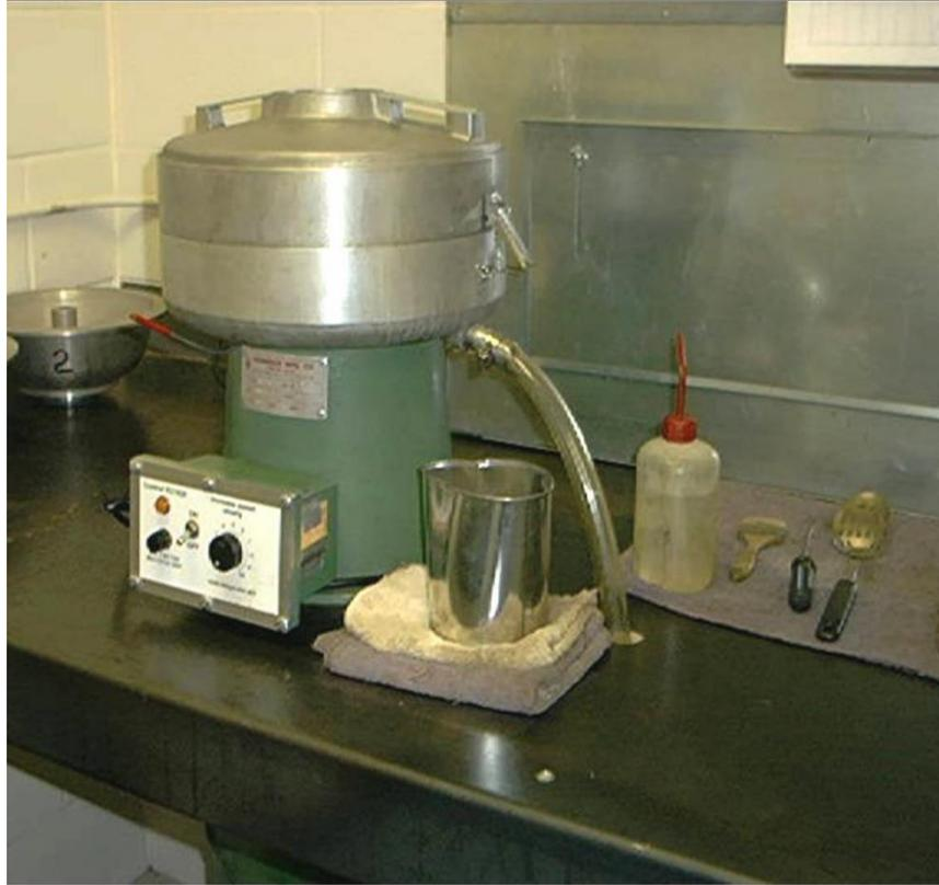
**Figure 700.6** – Centrifuge Extractor
