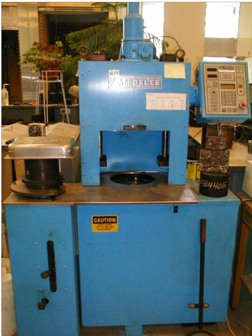
**Figure 700.5** – Gyrotory Compactor
