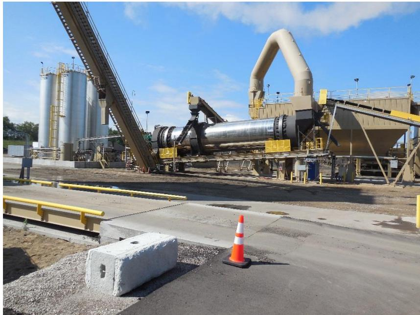
**Figure 400.1** – Dryer-Drum Asphalt Plant
