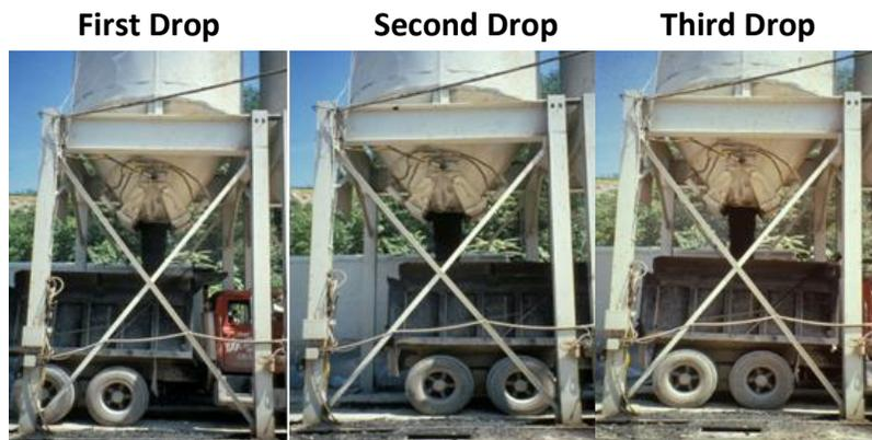
Figure 600.4 – Proper truck loading sequence
