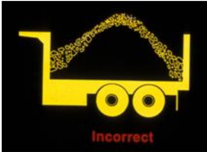
Figure 600.3 – Incorrect loading of asphalt mixture.
