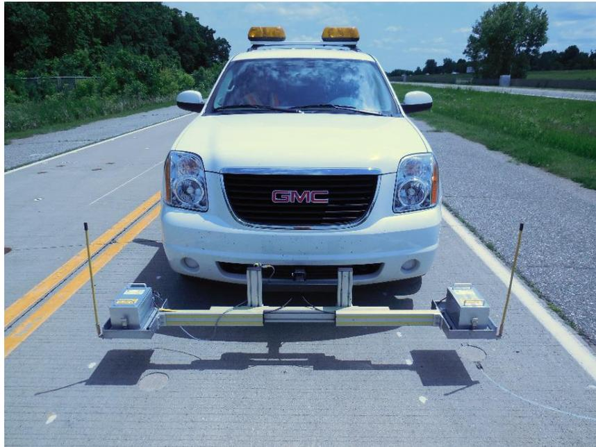
**Figure 500.29** – Inertial Profiler
