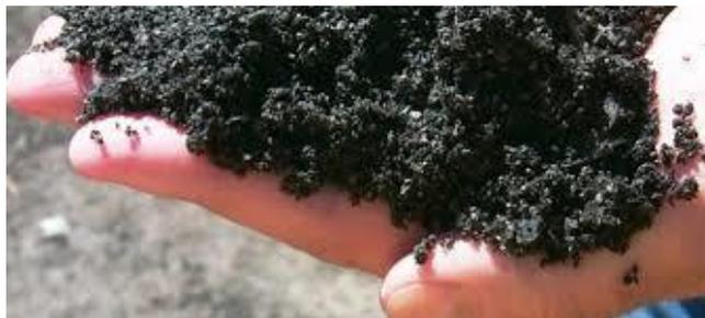
Figure 200.13 – Recycled Asphalt Shingles
